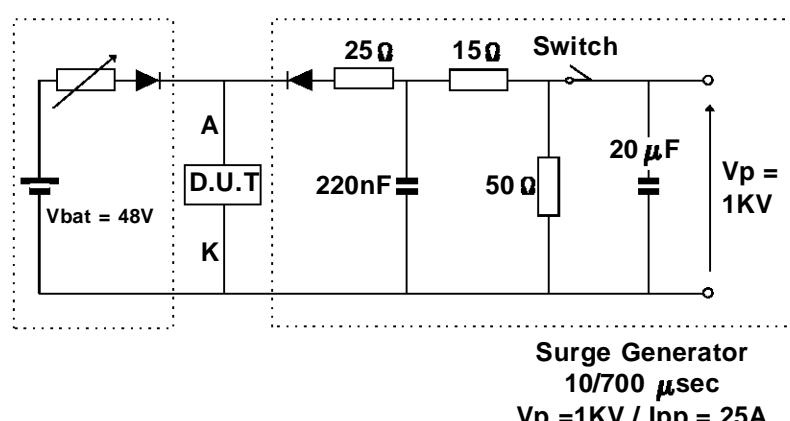
This test circuit performs a GO-NOGO test on the holding current  $I_H$ .
